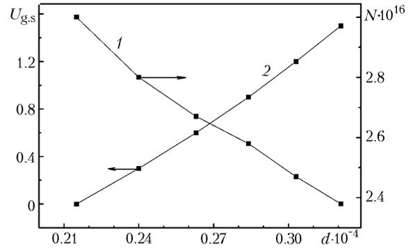
Fig. 4. Majority carrier density distribution in the base thickness (1) and depletion part of the base versus the cutoff voltage of the gate  $p$ - $n$  junction (2).  $U_{g,s}$ , V;  $d$ , cm;  $N$ ,  $\text{cm}^{-3}$ .
