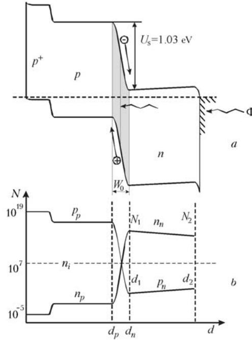
Fig. 5. Band structure of the  $p^+$ - $p$ - $n$  junction in the equilibrium state (a) and density distribution of carriers in the thickness (b).
