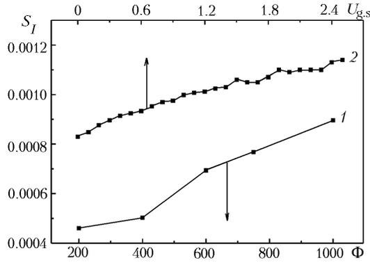
Fig. 10. Photosensitivity versus the cutoff voltage at 1000 lx (1) and the illumination intensity at a cutoff voltage of 0.3 V (2).  $S_I$ ,  $\mu\text{A}/\text{lx}$ ;  $\Phi$ , lx;  $U_{g,s}$ , V.
