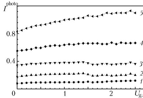
Fig. 8. Gate photocurrent versus the cutoff voltage at various integral illumination intensities: 1) 200 lx; 2) 400; 3) 600; 4) 800; 5) 1000.  $I^{\text{photo}}$ ,  $\mu\text{A}$ ;  $U_{g,s}$ , V.
