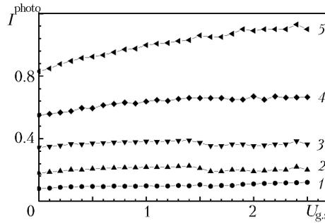
Fig. 8. Gate photocurrent versus the cutoff voltage at various integral illumination intensities: 1) 200 lx; 2) 400; 3) 600; 4) 800; 5) 1000.  $I^{\text{photo}}$ ,  $\mu\text{A}$ ;  $U_{g,s}$ , V.
