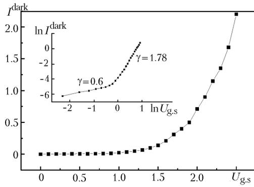
Fig. 3. Dark current of the gate  $p$ - $n$  junction as a function of the cutoff voltage (in the inset on a double logarithmic scale).  $I^{\text{dark}}$ ,  $\mu\text{A}$ ;  $U_{g,s}$ , V.
