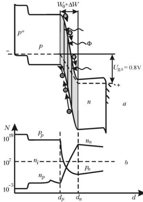
Fig. 9. Band structure of the  $p^+-p-n$  junction at a cutoff voltage of 0.8 V (a) and density distribution of carriers in the thickness (b).
