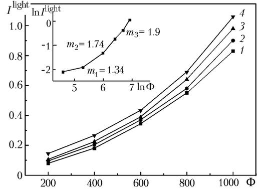
Fig. 7. Light current of the gate versus the illumination intensity at cutoff voltages of 1) 0 V; 2) 0.3; 3) 0.8; 4) 1.2.  $I^{\text{light}}$ ,  $\mu\text{A}$ ;  $\Phi$ , lx.
