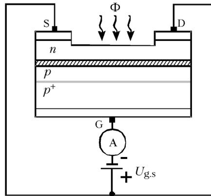
Fig. 2. Structure of the investigated GaAs field-effect phototransistor with a control  $p^+-p-n$  junction in the photodiode switching regime with connected drain and source leads; S, source; G, gate.
