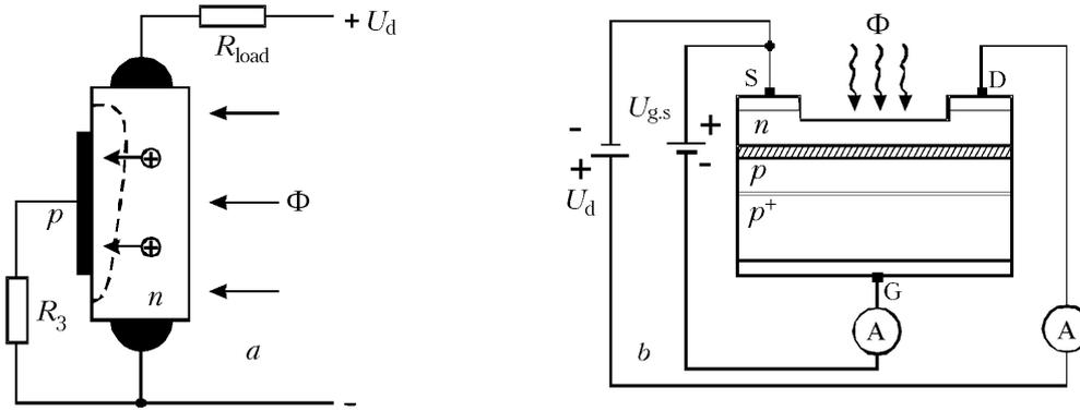
Fig. 1. Switching circuit of the field-effect phototransistor with self-bias on the gate [1] (a) and with a common source [3] (b); D, drain; S, source; G, gate.
