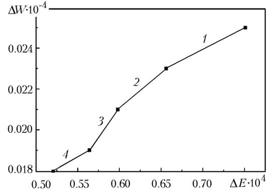
Fig. 11. Thickness increment of the space-charge layer versus the electric field strength increment of the gate  $p$ - $n$  junction as a junction of the given fixed voltages with a step of 0.3 V.  $\Delta E \cdot 10^4$ , V/cm;  $\Delta W \cdot 10^{-4}$ , cm.
