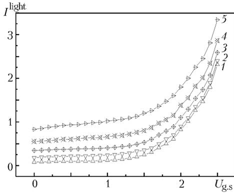
Fig. 6. Light current of the gate versus the cutoff voltage at various integral illumination intensities: 1) 200 lx; 2) 400; 3) 600; 4) 800; 5) 1000.  $I^{\text{light}}$ ,  $\mu\text{A}$ ;  $U_{g,s}$ , V.
