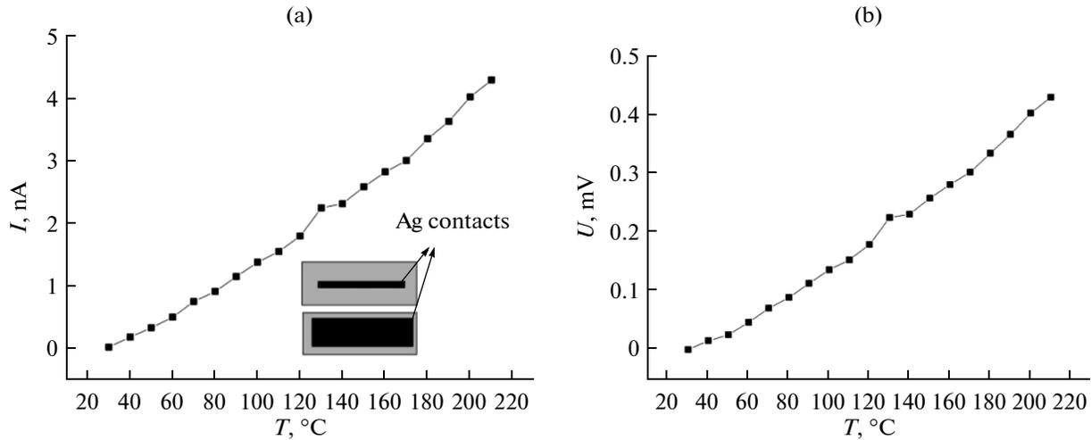
**Fig. 3.** Current (a) and voltage (b) as functions of temperature for  $n$ -type GaSb(Te) specimen with ohmic contacts. Schematic view of a specimen is illustrated in Fig. 3a.
