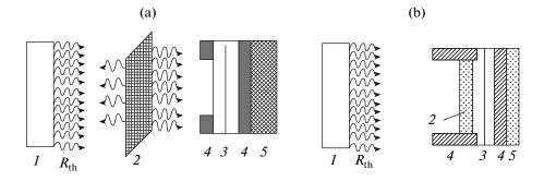
**Fig. 1.** (a) Main parts of a thermophotovoltaic facility: (1) thermal radiation source; (2) selective emitter (or reflector – filter); (3) photoelectric cell, p-n junction; (4) ohmic contacts; (5) radiator; (6) thermal radiation,  $R_{\text{th}}$ . (b) Parts of a thermophotothermovoltaic facility: (1) thermal radiation source; (2) photothermoelectric cell–transparent heat insulation layer; (3) p-n junction; (4) ohmic contacts; (5) heat insulation layer.
