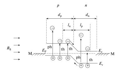
**Fig. 2.** Schematic diagram illustrating the band structure at the p-n junction of a photothermoelectric cell: M are metallic contacts; ph and th are photo- and thermoexcitation of eh pairs, respectively;  $l_n$  and  $l_p$  are diffusion paths of electrons and holes, respectively;  $d_n$  and  $d_p$  are widths of the *n* and *p* layers, respectively;  $R_S$  is solar radiation.
