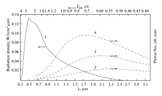
Fig. 3. (1) Spectral distribution of the solar radiation at the sea level in the case of clear sky; (2-4) photon flux densities for blackbody radiation corresponding to 1300, 1500, and 1700 K, respectively.
