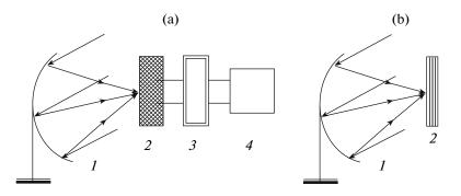
Fig. 4. Layouts of (a) solar power facility for the solar energy conversion to electricity: (1) concentrator of solar radiation; (2) receiver that converts solar radiation to heat; (3) heat engine; (4) electric power generator and (b) facility for converting concentrated solar radiation to electricity through the use of photothermoelectric cell: (1) concentrator; (2) photothermoelectric cell.
