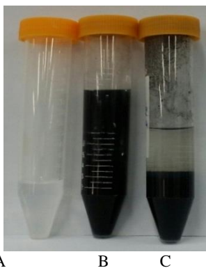
Figure 1. Prepared Dowtherm basic oil (A) and nanofluids: B –with 0.063 % 30 nm carbon, C- with 1% 30 nm carbon nanoparticles pictures.
